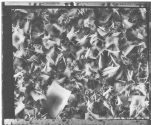
Fig. 7. Electron micrograph ( \times 600 ) of a cadmium electrode stored for 56 days at +60^\circ\text{C} in 6 M KOH containing 0.1% turkey red oil.
